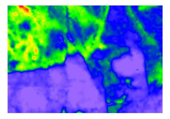
Ground Conductivity Mapping is one of the most cost effective Geophysical methods available. Rapid acquisition is made possible using custom vehicle setups (using a 4WD or ATV). Ground conductivity and position data are logged continuously in real-time whilst driving, making it possible to cover many hectares in one day. Applications for conductivity mapping include:
